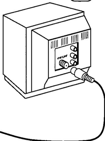
**2** Connect the VCR to your TV with the RF Coaxial Cable (OUT TO TV).
