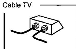
**1** Disconnect the antenna or cable from your TV and connect it to the VCR (IN FROM ANT.)
