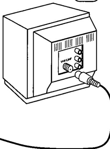
RF Coaxial Cable (VCR-TV Connection Cable) (supplied)
