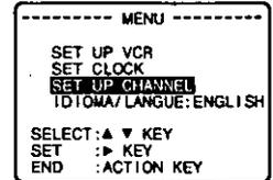
**2** Press ▲▼ to select "SET UP CHANNEL," and then press ► to display the "SET UP CHANNEL" screen.
