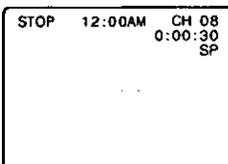
**b** Press **COUNTER RESET** to reset the Time Counter to "0:00:00" at the desired position.
