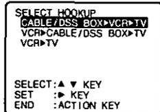
**5** Press ▲▼ to select your cable box or DSS receiver output channel number, and then press ▶ to enter.
