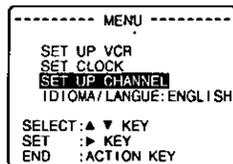
**2** Press ▲▼ to select "SET UP CHANNEL," and then press ► to display the "SET UP CHANNEL" screen.
