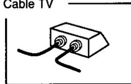
**1** Disconnect the antenna or cable from your TV and connect it to the VCR (IN FROM ANT.)
