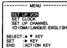
**2** Press ▲▼ to select "SET UP VCR," and then press ▶ to display the "SET UP VCR" screen.
