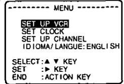
**2** Press ▲▼ to select "SET UP VCR," and then press ► to display the "SET UP VCR" screen.
