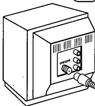
RF Coaxial Cable (VCR-TV Connection Cable) (supplied)
