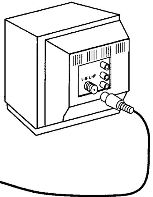
RF Coaxial Cable (VCR-TV Connection Cable) (supplied)
