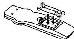
**3** Fit the lid's hinge piece into the indent on the case, and snap the lid into place.
