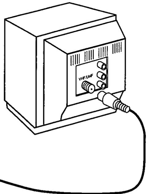
RF Coaxial Cable (VCR-TV Connection Cable) (supplied)
