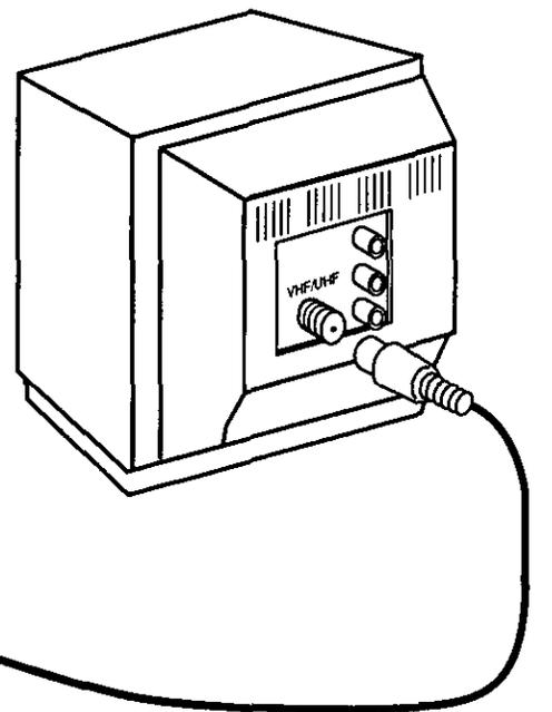
RF Coaxial Cable (VCR-TV Connection Cable) (supplied)
