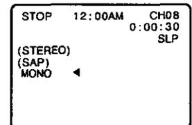
b Push COUNTER RESET to reset the Time Counter to "0:00:00."
