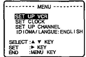
② Push ▲▼ to select "SET UP VCR," and then push ► to display the "SET UP VCR" screen.
