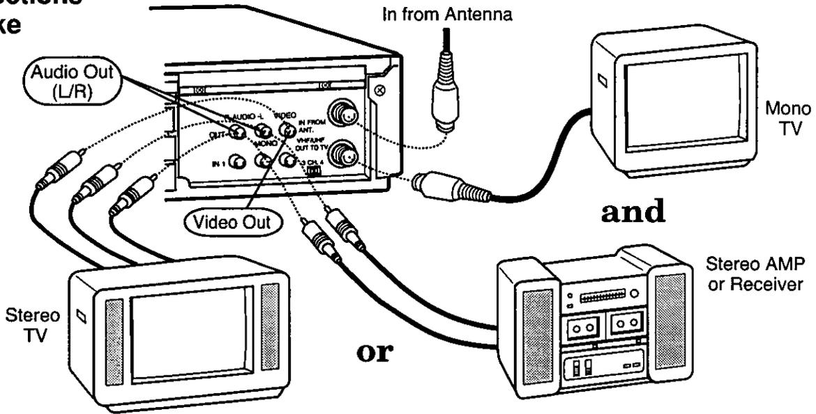
When recording, you may monitor in stereo, by connecting the VCR to either a stereo TV, or a mono sound TV with an external stereo amp and speakers.
