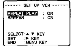
The VCR plays back the tape to its end or until a blank portion of over 30 seconds is detected (erased portions are not considered blank). The tape is then rewound and played again and again until Repeat Play is turned off.
