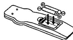
**3** Fit the lid's hinge piece into the indent on the case, and snap the lid into place.
