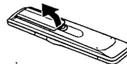
**2** Install three batteries as indicated inside the Battery Compartment.
