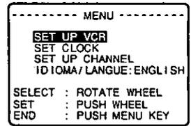
② Rotate and push the WHEEL to select SET UP VCR.
