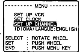
**b** Rotate and push the WHEEL to select SET UP CHANNEL.
