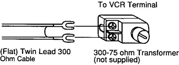
**Case 2: Twin Lead & Coaxial Cables**
