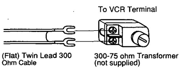
**Case 2: Twin Lead & Coaxial Cables**
