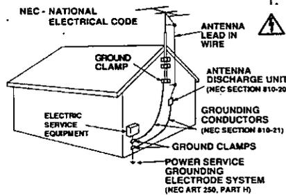
1. INSURE SAFE ANTENNA AND CABLE CONNECTIONS. If an outside antenna or cable system is connected to the equipment, be sure the antenna or cable system is grounded so as to provide some protection against built up static charges and voltage surges. Part 1 of the Canadian Electrical Code, in USA Section 810 of the National Electrical Code, ANSI/NFPA
