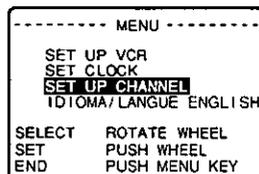
2 Rotate and push the WHEEL to select SET UP CHANNEL
