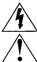
This symbol warns the user that uninsulated voltage within the unit may have sufficient magnitude to cause electric shock. Therefore, it is dangerous to make any kind of contact with any inside part of this unit.
