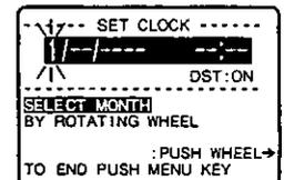
2 Rotate and push the Wheel to select and enter the month, date, year, time and D.S.T. (Daylight Saving Time).
