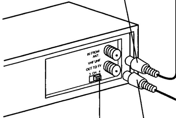
Set the Output Channel of your VCR to channel 3 or 4 (whichever is not being transmitted on by a Local TV broadcast).
