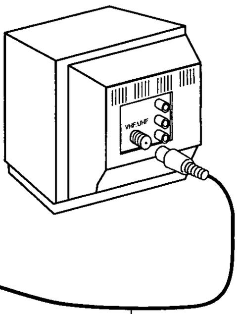
RF Coaxial Cable (VCR-TV Connection Cable) (supplied)
