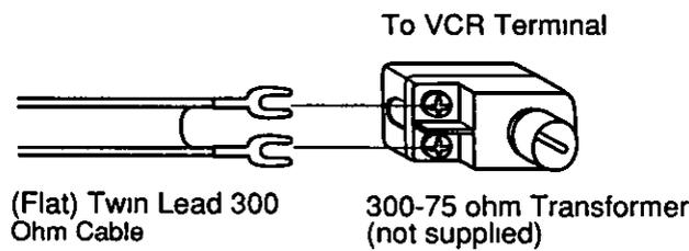
**Case 2: Twin Lead & Coaxial Cables**
