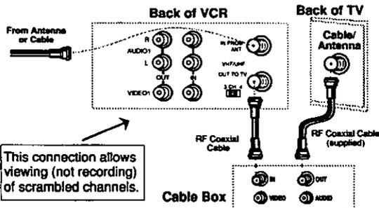
This connection allows viewing (not recording) of scrambled channels.
