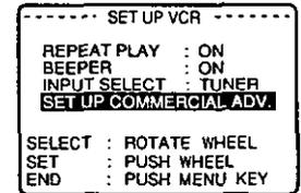
③ Rotate and push the WHEEL to select SET UP COMMERCIAL ADV.
