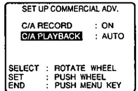
**AUTO** The VCR will automatically advance through marked commercial blocks recorded on the tape and then resume playback.
