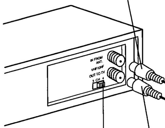
Set the Output Channel of your VCR to channel 3 or 4 (whichever is not being transmitted on by a Local TV broadcast).
