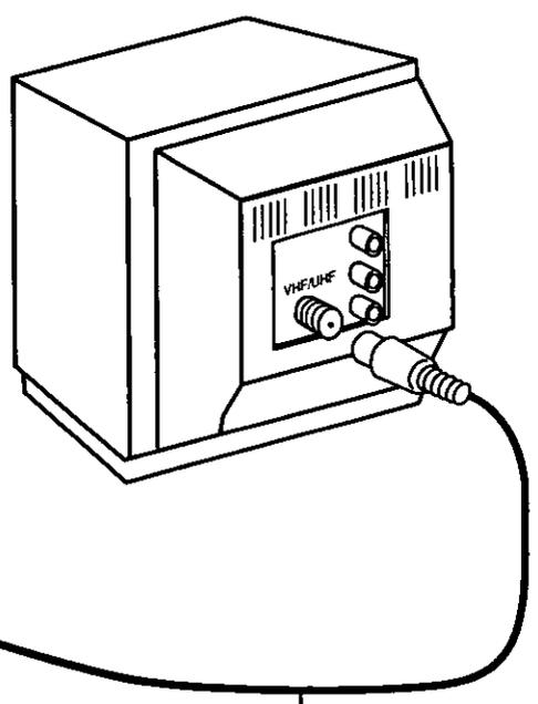
RF Coaxial Cable (VCR-TV Connection Cable) (supplied)
