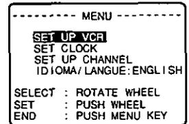
② Rotate and push the WHEEL to select and set SET UP VCR from the menu screen.
