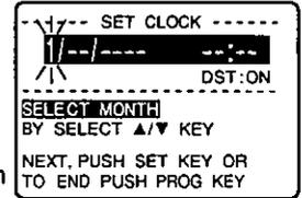
• If the clock is not set, pushing these buttons will display the SET CLOCK screen. In this case, proceed with steps 2 and 3 to set the clock and then steps 2~6 to set a timer recording.
