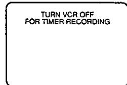
If you Push REC on the remote control or REC and PLAY on the VCR, and a cassette is inserted with no record tab...
