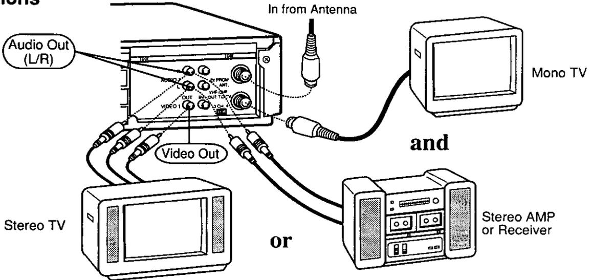
When recording, you may monitor in stereo, by connecting the VCR to either a stereo TV, or a mono sound TV with stereo amp and speakers.
