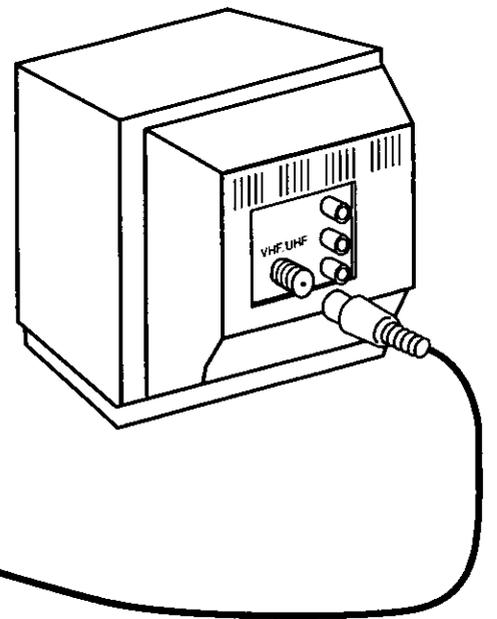
RF Coaxial Cable (VCR-TV Connection Cable) (supplied)
