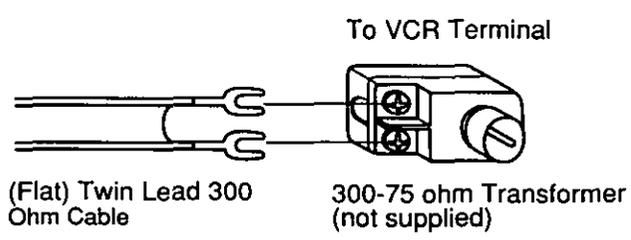
**Case 2: Twin Lead & Coaxial Cables**
