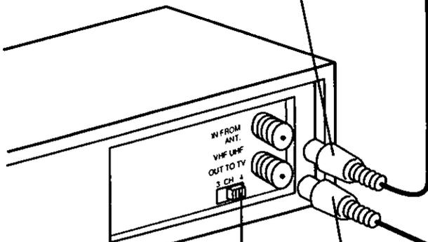
Set the Output Channel of your VCR to channel 3 or 4 (whichever is not being transmitted on by a Local TV broadcast).
