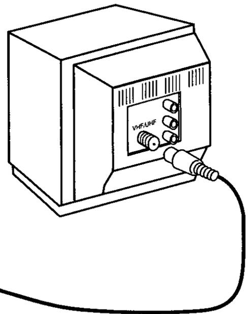
RF Coaxial Cable (VCR-TV Connection Cable) (supplied)
