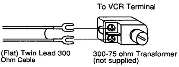
**Case 2: Twin Lead & Coaxial Cables**
