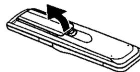
**2** Install two batteries as indicated inside the Battery Compartment.
