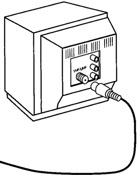
RF Coaxial Cable (VCR-TV Connection Cable) (supplied)
