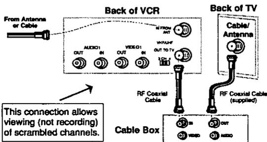
This connection allows viewing (not recording) of scrambled channels.
