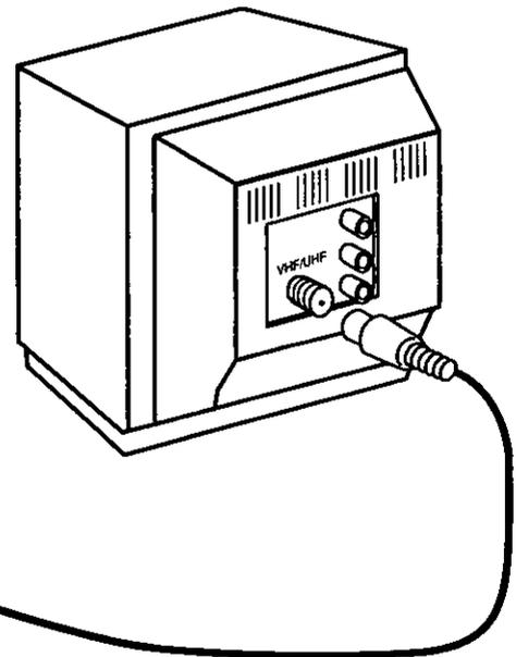
RF Coaxial Cable (VCR-TV Connection Cable) (supplied)
