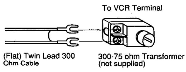
**Case 2: Twin Lead & Coaxial Cables**
