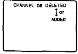
• To select a deleted channel, use the NUMBERED keys on the remote control. Deleted channels will flash in the Multi Function Display on the VCR when selected.
