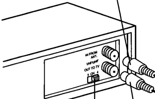
**Set the Output Channel of your VCR to channel 3 or 4 (whichever is not being transmitted on by a Local TV broadcast).**
