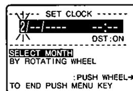
⑦ Rotate and push the WHEEL to set remaining items at right.
