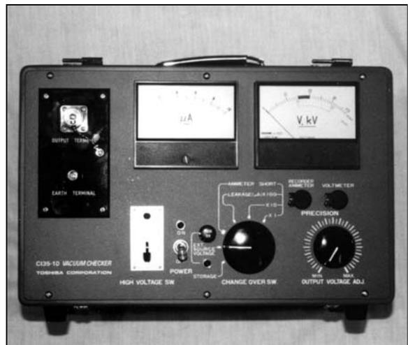
**Fig. 32 Toshiba Portable Vacuum Checker**
