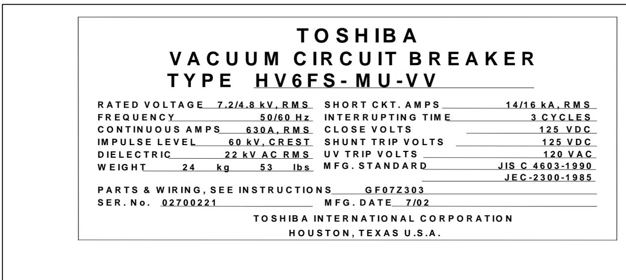
Fig. 8 Typical Circuit Breaker Nameplate
