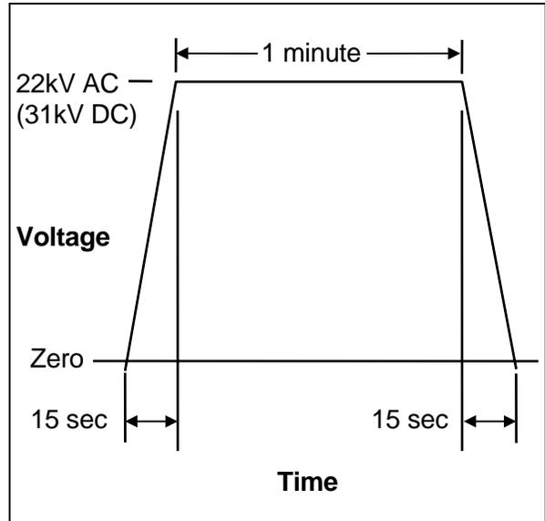
Fig. 33 Application of Test Voltage for Vacuum Check
