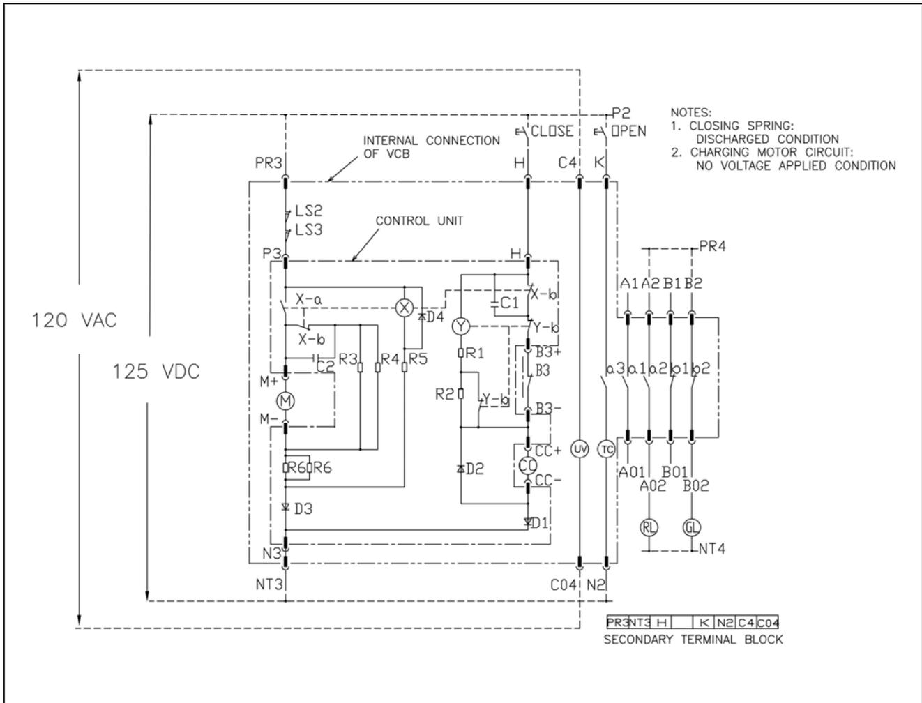
Fig. 28 125 VDC Control Circuit Schematic for MU Type Circuit Breaker
