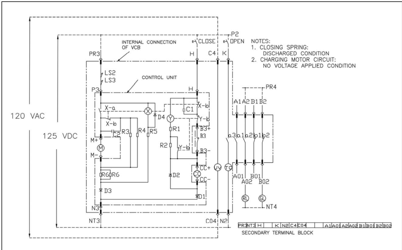
Fig. 29 125 VDC Control Circuit Schematic for ML Type Circuit Breaker
