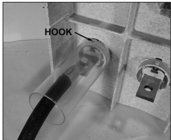
**Fig. 17 Fasten Insulating Cylinder**
