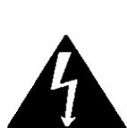
The lightning flash with arrow-head within a triangle is intended to tell the user that parts inside the product are a risk of electric shock to persons
