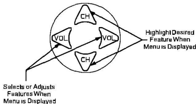
**Favorite Channel Select** – The Favorite Channel Programming feature allows you to program up to 15 of your favorite channels into your personal channel scan memory. Use the CH buttons on the Remote Control to scan channels without going through channels you don't normally view. Favorite Channel will effect both regular channel selection and PIP Channel selection.
