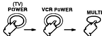
To delete entered functions – Press the Remote TV POWER and MULTI buttons simultaneously Now you can enter from one to six different Remote functions
