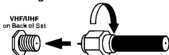
**Cable Connection** – For reception of cable channels (01–125) connect the cable supplied by your local cable company. Antenna Mode must be set to CABLE (Refer to Antenna Mode section)
