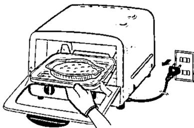
After using, unplug the power plug from the wall outlet.
