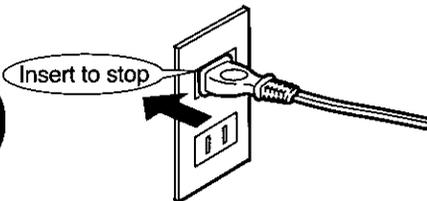
If the plug is inserted improperly it may cause electric shock or generate heat resulting in fire.
