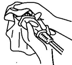
A build-up of dust on the plug will attract condensation, which could cause cable damage resulting in fire.
