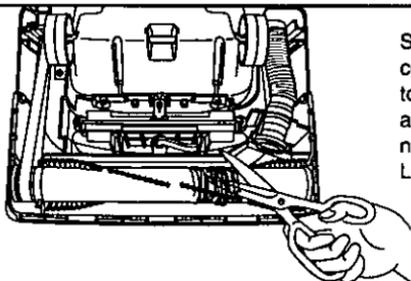
Switch off the vacuum cleaner and unplug the power cord before cleaning the agitator assembly. In order to keep the cleaning efficiency high, clean the agitator assembly regularly. Remove the lower plate if necessary. See the REMOVING/INSTALLING THE LOWER PLATE section for the proper procedure.
