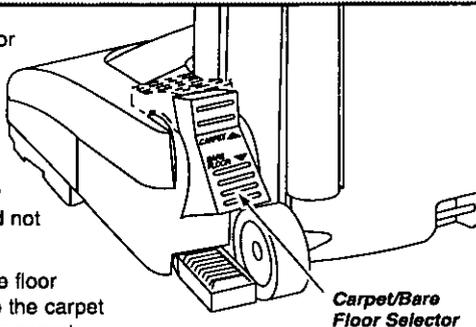
To use cleaner on carpeted areas, the carpet/bare floor selector should be **all the way forward** and up to the carpet position. This will allow the agitator to turn. When carpets are being cleaned the selector should remain in this position.
