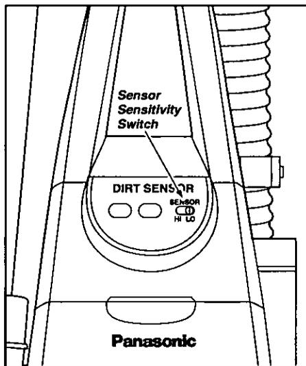
Even with the sensor switch in the LO position, the dirt sensor will detect carpet fuzz, especially on new carpet, which may cause the red light to remain on longer than expected.
