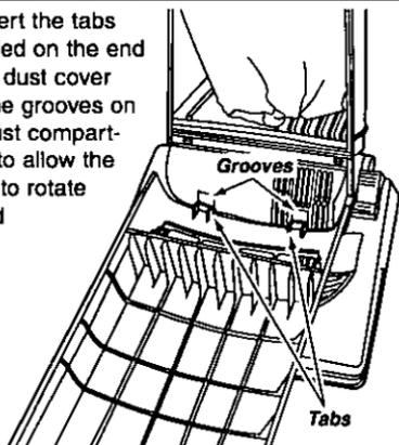
**Note** The dust cover must be completely and correctly installed for proper operation
