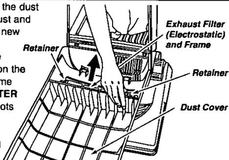
**This filter cannot be cleaned and should be replaced at least once each year if the cleaner is used at least one hour each week.**
