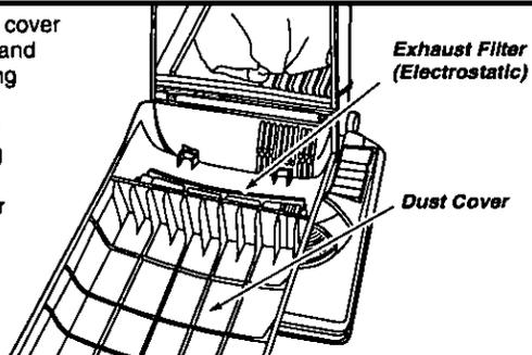
**This filter cannot be cleaned and should be replaced at least once each year if the cleaner is used at least one hour each week.**
