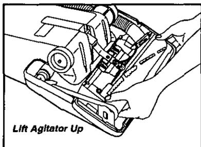
Unplug and turn the unit over. Remove the lower plate as described in the Removing/Installing the Lower Plate section. Remove the agitator brush assembly (carefully lift it out), and remove the worn or broken belt from the agitator pulley and motor drive shaft.
