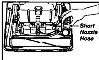
Remove the lower plate Remove the short nozzle hose from the housing by lifting it straight up Inspect the hose end and clear it of any obstructions Reinstall the short nozzle hose and lower plate See the Removing/Installing the Lower Plate section for detailed instructions
