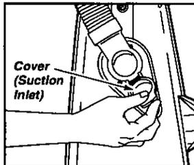
Pull down on the suction inlet cover and check for clogging in this area
