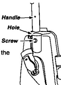
2. Line up the small hole in the handle with the small hole in the vacuum cleaner and insert the screw that you have removed. Use a screwdriver to assure the screw is tightened securely.
