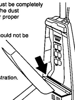
6. Reinsert the tab provided on the end of dust cover into the groove on the dust compartment and press the cover into place.
