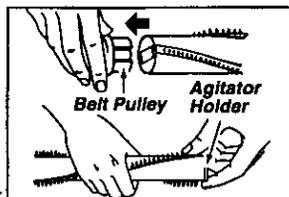
**Note** Take care not to bend the agitator shaft. Do not misplace the small E-clip. Be careful when removing and reinstalling it from the shaft end, as it can easily get away from you.
