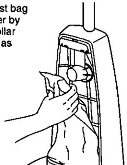
5. The dust bag must be completely installed inside the dust compartment for proper operation.
