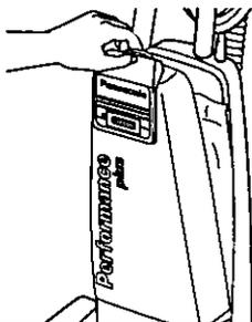
2. To remove the dust bag, grasp the cardboard portion of dust bag and pull it out.
