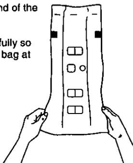
4. Attach the new dust bag onto the bag holder by holding the bag collar and pushing back as illustrated.
