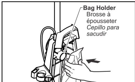
➤ Attach new dust bag onto bag holder by holding cardboard portion and pushing back.
