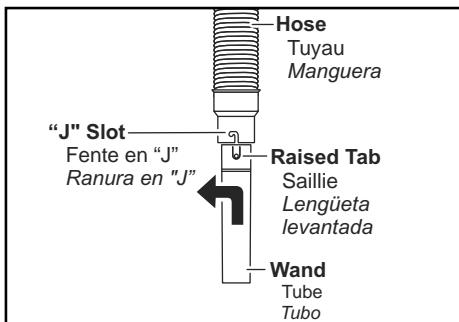
➤ Attach wand to hose by aligning the two (2) raised tabs on wand with "J" slots in hose, guide tabs along grooves, twist to lock in place.
