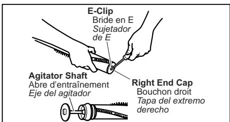
➤ Remove lower plate and agitator.
