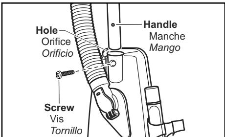
➤ Insert handle with cord hook to the back of the vacuum cleaner.
