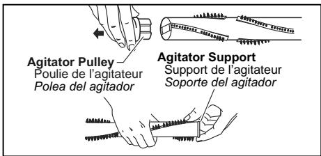
➤ Remove the E-clip from agitator shaft and end cap.
