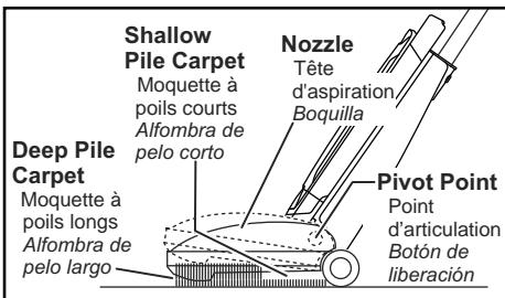
➤ The nozzle of your Panasonic vacuum cleaner automatically adjusts to any carpet pile height.
