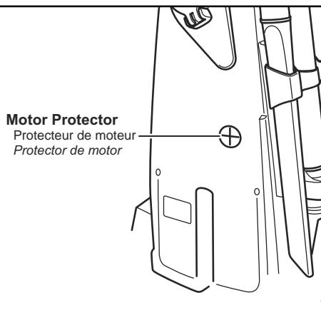
➤ The motor protector automatically opens to provide cooling air to the motor when a clog occurs or when dust bag needs changing.
