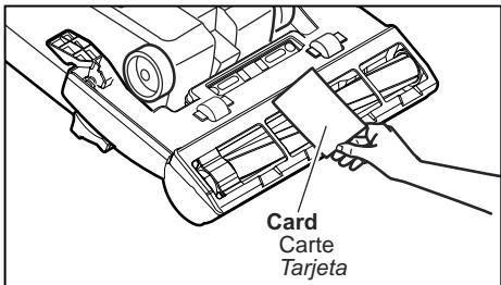
➤ When the bristles on the agitator are worn so that they do not touch a card held across the lower plate, the brushes should be replaced.
