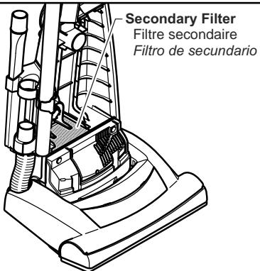
➤ Secondary filter protects the motor.
