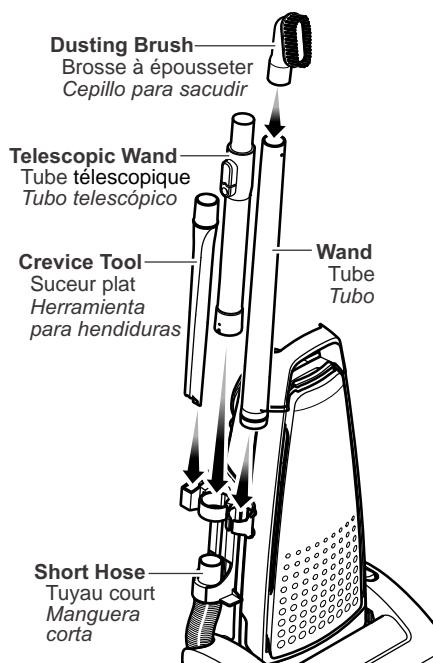
➤ Place wand in center slot of tool holder, twisting and pushing down over short hose to assure a good connection.
