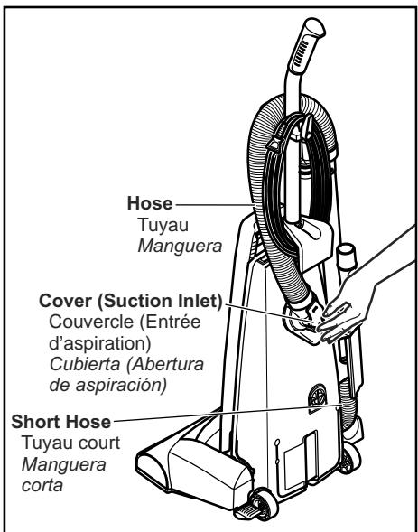
The hose located on the back of the vacuum cleaner carries the dirt from the nozzle up to the dust bag. If the hose should become clogged:
