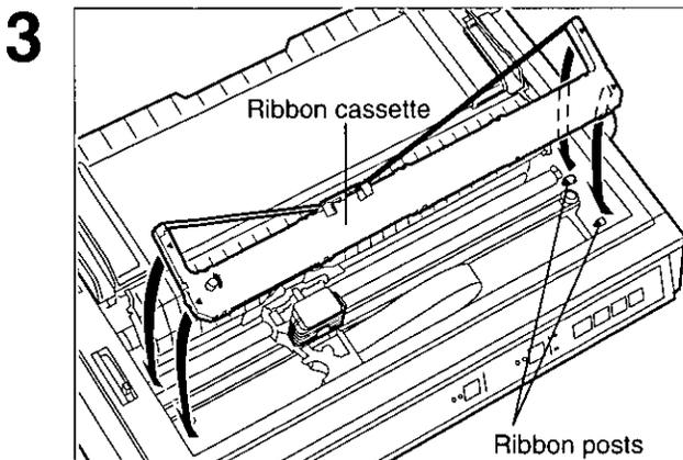
Lower the ribbon cassette onto the four ribbon posts (gold in color), insert the back portion of the ribbon into the printer first.
