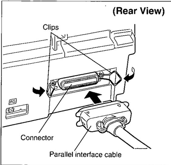
Attach the other end of the parallel interface cable from your computer to your printer and secure the printer clips.
