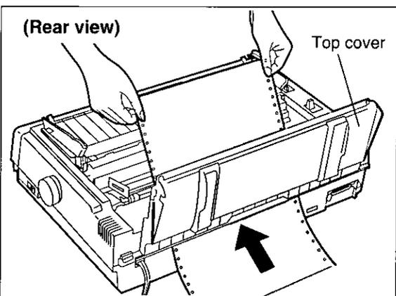
Feed paper through opening between printer and the top cover.
