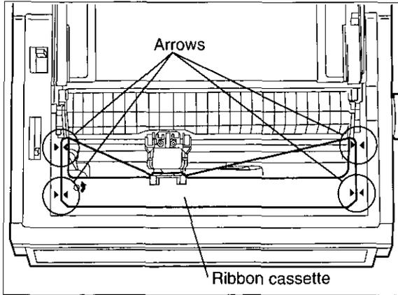
Line up the 4 arrows on the ribbon cassette with the arrows on the left and right sides of the frame. Push 4 arrows down until they click into place.
