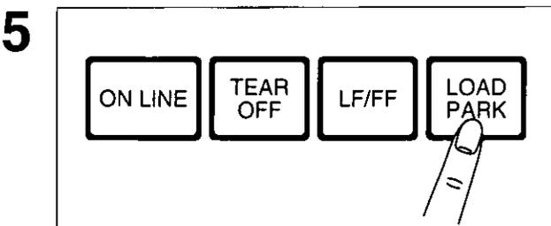
Press **LOAD/PARK** to reload the fanfold paper to the first print line.
