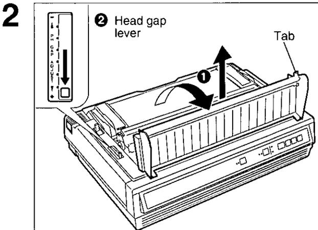
**1 Raise the smoked plastic cover using the tab and remove it.**
