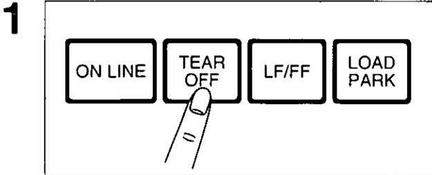
Press **TEAR OFF** to advance the paper to the tear bar.
