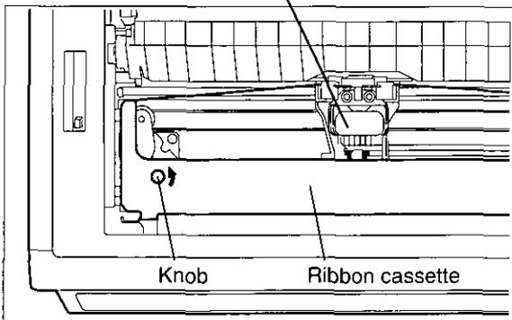
Rotate the knob on the ribbon cassette counterclockwise to remove any slack.
