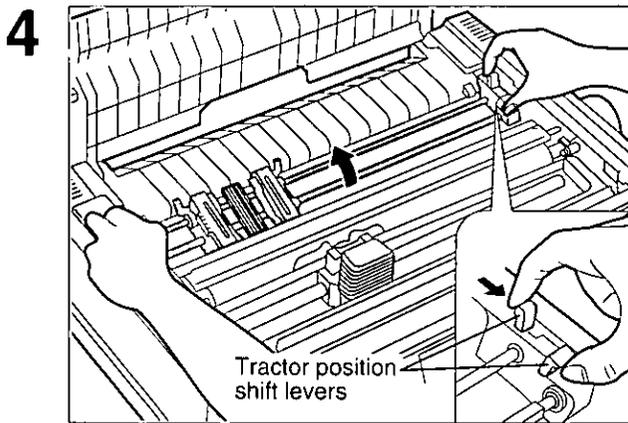
Pinch both left and right tractor position shift levers, and lift the tractor mechanism up then release the levers.
