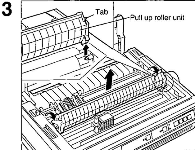
Remove the pull up roller unit by grabbing the tabs at both ends and gently rotating forward until you feel it release, then lift up.
