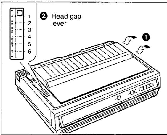
② Adjust the head gap lever for the thickness of paper you are using.
