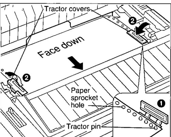
① Align the paper sprocket holes with the tractor pins, making sure the paper is straight.
