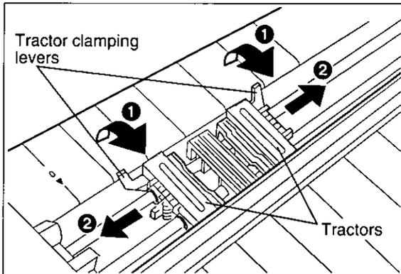
① Unlock the tractors by pulling the tractor clamping levers forward.
