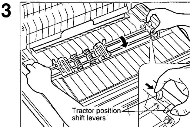
Pinch both left and right tractor position shift levers and lower the tractor mechanism downward until the tractors fall into place, then release.
