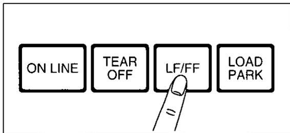
With paper installed, holding **LF/FF** moves the printhead to the center and advances the paper to the top of the next page.
