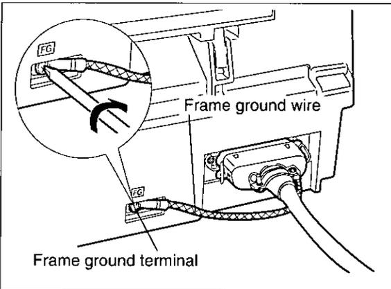
If the cable has a frame ground wire, connect it to the frame ground terminal.
