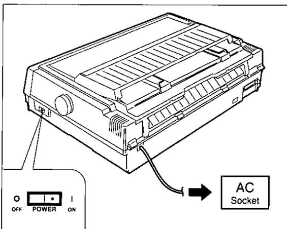
Plug printer into a grounded 3 prong AC socket.
