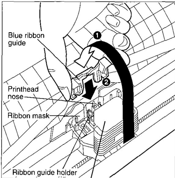
① Grasp the top of the blue ribbon guide with your thumb and forefinger, remove the blue ribbon guide by lifting from the ribbon cassette.
