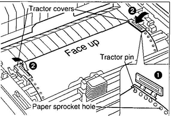
1 Align the paper sprocket holes with the tractor pins, making sure the paper is straight.
