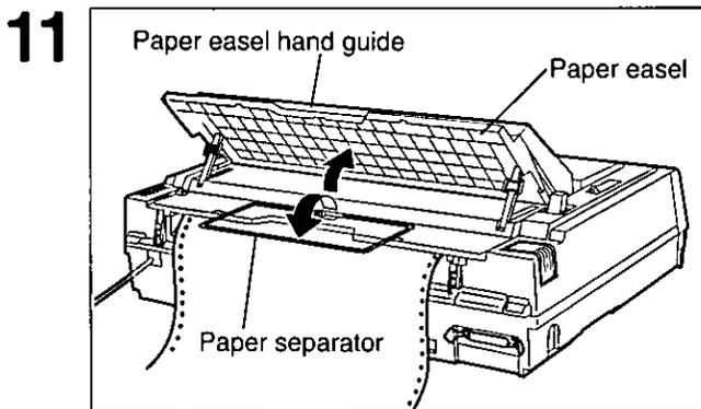
Extend the paper separator by first raising the paper easel by lifting the paper easel hand guide and then unfolding it.
