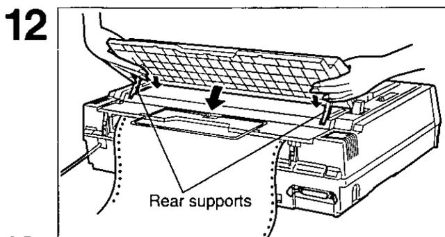
Lower the paper easel by simultaneously depressing the rear supports.
