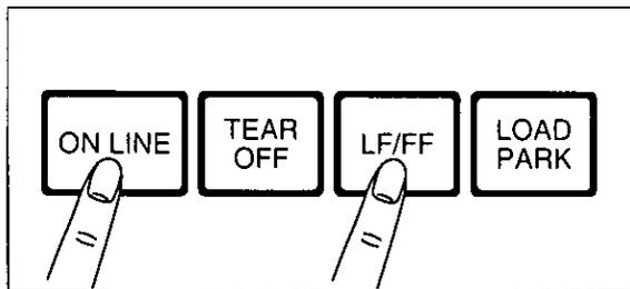
With paper installed, while pressing **ON LINE**, press **LF/FF** once to advance the paper one micro line ( $\frac{1}{216}$ ""). Holding the switches will advance the paper continuously until you release the switches. Using the Micro Line Feed within 5" from the top of your paper automatically stores the position as the Top of Form.
