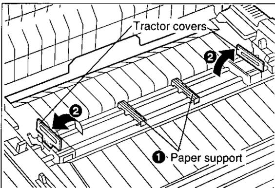
① Slide the two paper supports between the tractors at equal spaces.
