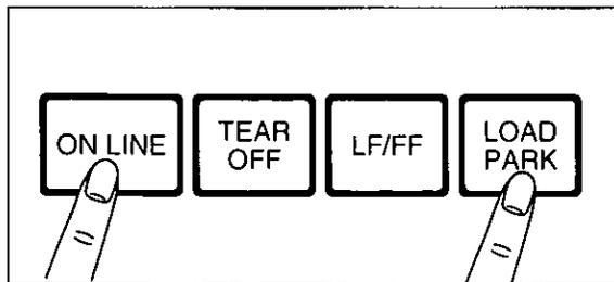
With paper installed, while pressing **ON LINE**, press **LOAD/PARK** once to reverse the paper one micro line ( $\frac{1}{216}$ ""). Holding the switches will reverse the paper continuously until you release the switches. Using the Reverse Micro Line Feed within 5" from the top of your paper automatically stores the position as the Top of Form.
