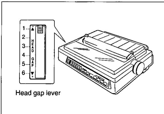
Adjust the head gap lever for the thickness of the paper you are using.
