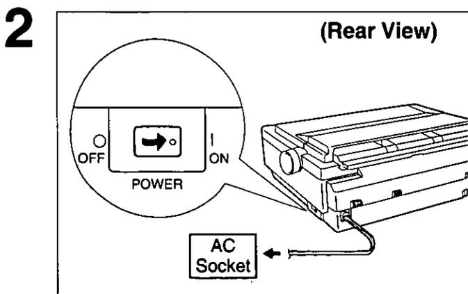
Plug the printer into a grounded 3 prong AC socket.
