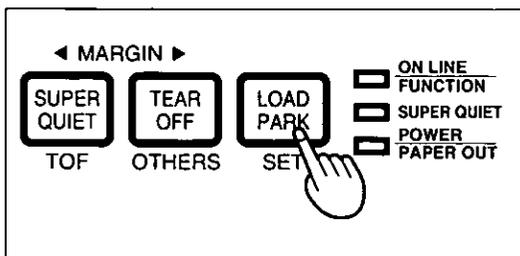
Press **LOAD/PARK** to reload the fanfold paper to the Top of Form.
