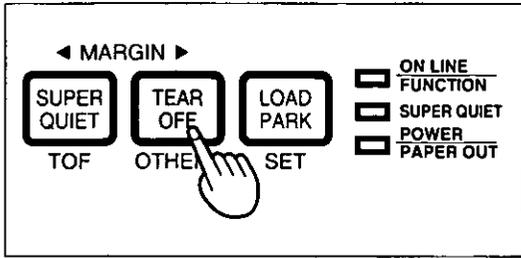
Press **TEAR OFF** to advance the paper's perforation to the tear bar.
