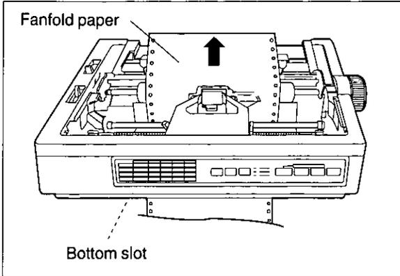
Push the fanfold paper up through the bottom opening until it appears on the platen.
