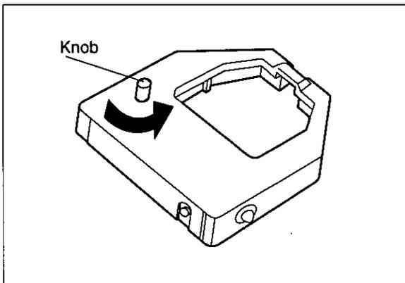
Rotate the knob on the ribbon cassette to remove any slack.
