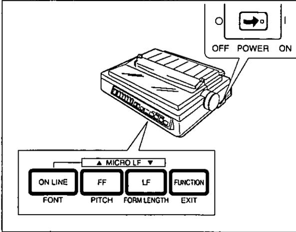
While pressing both **LF** and **FF**, turn the power on.
