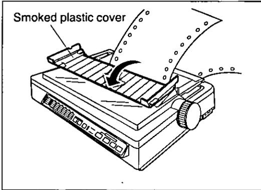
Fold the smoked plastic cover forward by lifting tab on right side.
