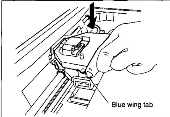
Press down on rear of the cassette until the blue wing tab snaps into place.
