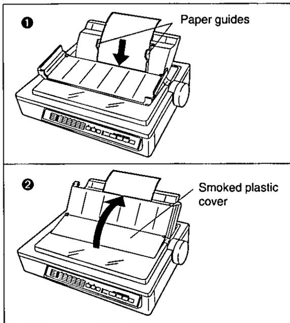
1 Insert a sheet of paper through the paper guides and behind the platen.
