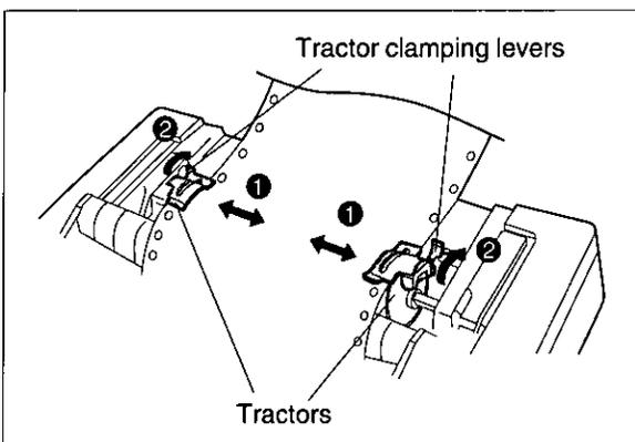
① Adjust the tractors to remove any slack from the paper.
