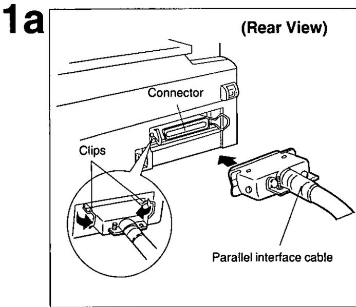
Attach one end of the parallel interface cable to your printer as shown, and the other end to your computer. Be sure to secure the printer clips.
