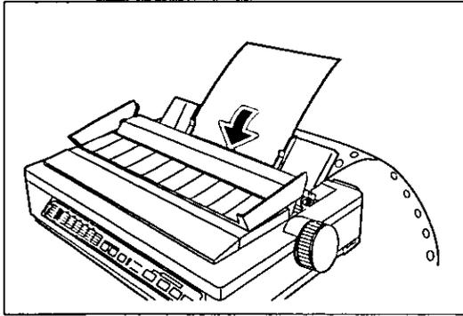
Separate the paper guides and load a single sheet or an envelope.
