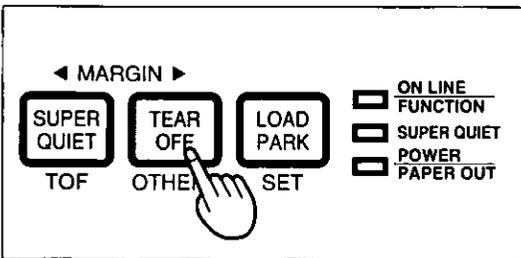
Press **TEAR OFF** to reverse the paper back to the Top of Form.
