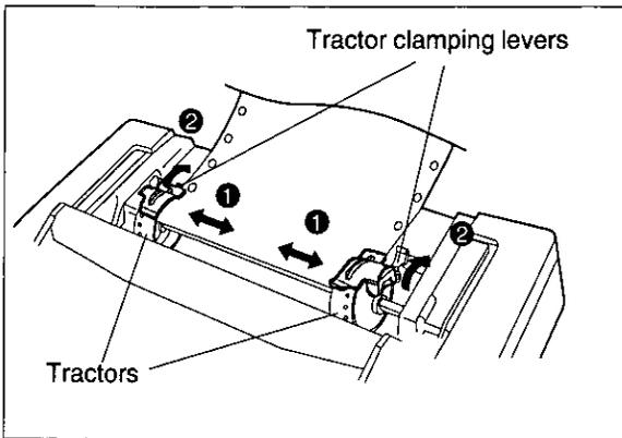
❶ Adjust the tractors to remove any slack in the paper.
