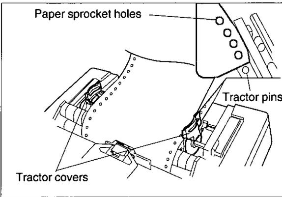
Align the paper sprocket holes with the tractor pins.
