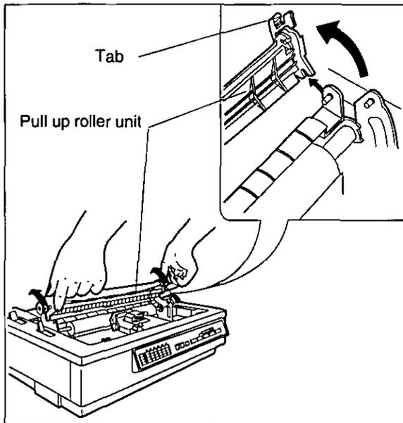
**Remove the pull up roller unit.**
