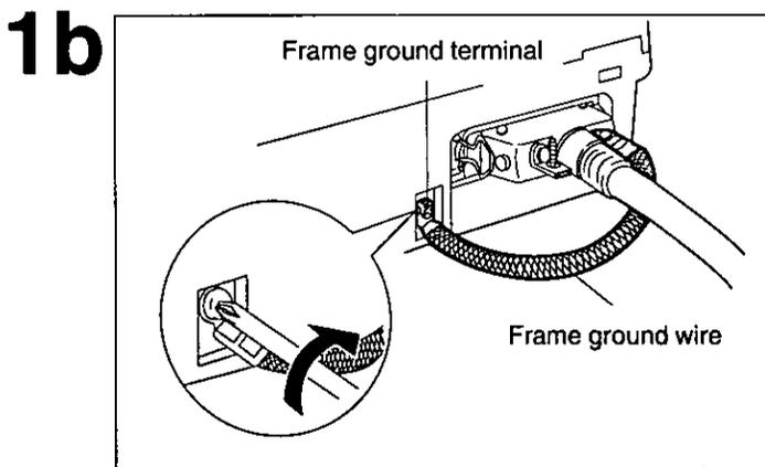
If the cable has a frame ground wire, connect it to the frame ground terminal.
