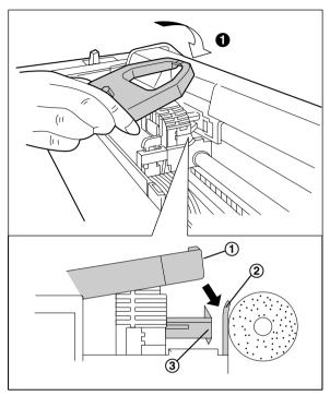
2 Press down on rear of the ribbon cassette until the wing tab (1) snaps into place.
