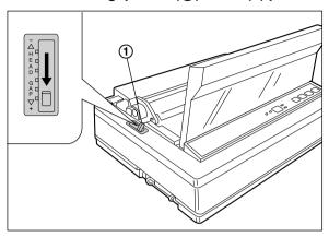
3. Rotate the knob (1) on the ribbon cassette to remove any slack.
