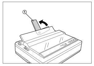
Insert a sheet of paper with the printed side face down behind the platen by aligning its left edge with on the top cover.
