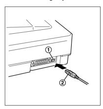
When connecting with a parallel interface cable: Attach the parallel interface cable (③) from your computer to the parallel interface connector (①) and secure the printer clips (②).
