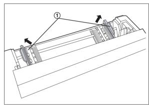
6. Place the paper with the printed side face down and align the paper sprocket holes with the tractor pins, then close the tractor covers.
