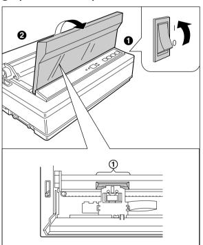
2. Move the head gap lever (1) to the (+) position.
