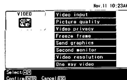
3. Select the One way video mode using the **▼** cursor key, and then press the **ENTER** key.
