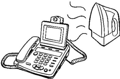
Do not place the unit in direct sunlight or near a cooling or heating (air-conditioning) unit. Using the unit at temperatures above 35°C or below 5°C can cause incorrect operation, deformation or malfunctioning.
