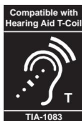
Telephone handsets identified with this logo have reduced noise and interference when used with T-Coil equipped hearing aids and cochlear implants.
