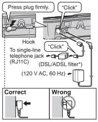
\*DSL/ADSL filter (not supplied) is required if you have DSL/ADSL service.
