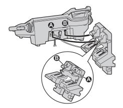
**3** Adjust the adaptor to hold the base unit, then push it in the direction of the arrow until it clicks into place.
