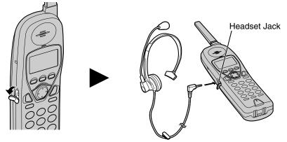
To switch to the speakerphone while using the headset: Press ∉ . To return to the headset, press ♠. Useful Information
