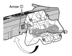
5 While keeping the adaptor held to the base unit, slide the wall mounting adaptor to the left until it clicks into place.
