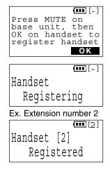
•You can stop registration by pressing **OFF** on the handset and pressing **MUTE** on the base unit.
