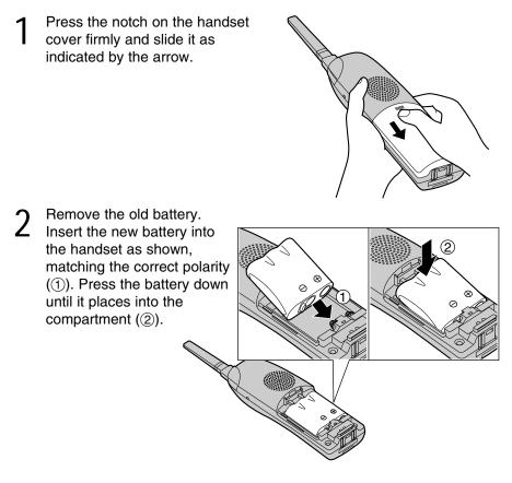
3 Close the cover. Make sure you charge the new battery for about 15 hours in order to display the battery strength prompt correctly (p. 12).
