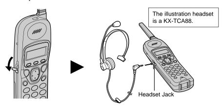
To switch to the speakerphone while using the headset:
