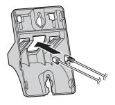
2 Tuck the telephone line cord inside the wall mounting adaptor (1). Connect the AC adaptor cord and telephone line cord (2).
