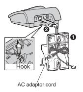
3 Insert the hooks on the wall mounting adaptor into the holes **a** and **3** on the base unit.
