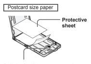
Pull the feeding stop upwards.
