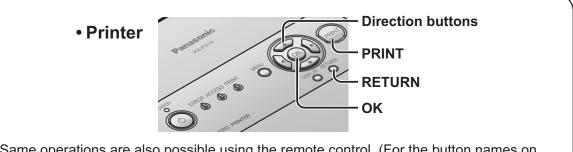
Same operations are also possible using the remote control. (For the button names on the remote control, refer to page 14.)
