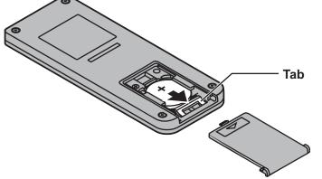
Pressing down on the tab, slide out the coin battery and remove.
