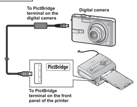
Connect the camera to the printer using the USB cable provided with the digital camera.
