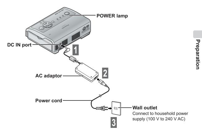
When the power cord is connected to wall outlet, the POWER lamp lights up in red (standby mode).
