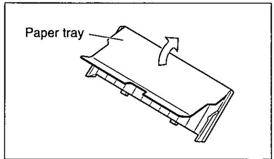
2 Insert the two fins on the paper tray into the slots on the back of the unit.
