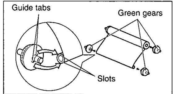
7 Insert the film into the cartridge so that the blue gear matches the blue label on the cartridge.
