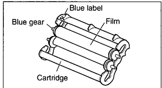
8 Lock the four gears of the film by (A) pushing back the top side gears and (B) pulling the bottom side gears forward until they lock into place.
