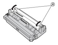
6 Make sure that the arrows (⑤) match to install the toner cartridge correctly.
