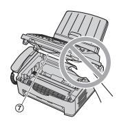
5 Clean the document feeder roller (®) with a cloth moistened with isopropyl rubbing alcohol, and let all parts dry thoroughly.
