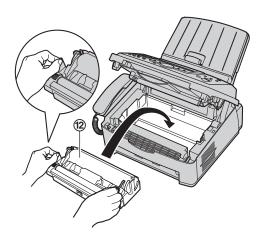
**10** Close the front cover (**(3)**) by pushing down on both sides, until locked.
