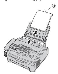
9 Attach the paper tray cover (4), then push back the tension plate (45).
