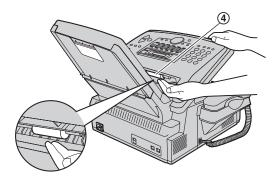
4 Hold the center part of the front cover (⑤), and pull open the inner cover (⑥).
