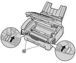
**7** Close the front cover (11) by pushing down on both sides, until locked.
