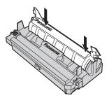
5 Turn the two levers (4) on the toner cartridge firmly.
