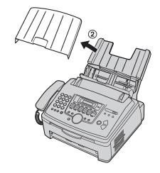
4 Pinch the right side of the recording paper guides (3), then slide it open to its full width.
