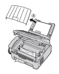
3 Remove the recording paper (⑤), then remove the drum and toner unit (⑥) to allow the jammed paper (⑦) to pull free from the rear cabinet.
