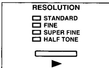
**STANDARD** is suitable for printed or typewritten originals with normal-sized characters.
