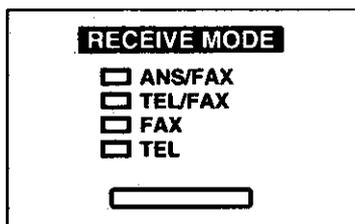
Press the **RECEIVE MODE** button to select the desired receiving mode.
