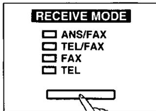
Press the **RECEIVE MODE** button until the ANS/FAX indicator lights.
