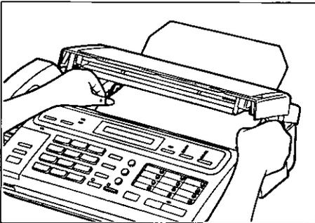
Replace the recording paper roll. Then insert its leading edge into the recording paper exit and pull the paper a few centimeters (one or two inches) out of the unit. Make sure that the shiny side of the paper is facing up and that there is no slack in the paper roll.
