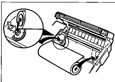
Insert the left projection of the paper roll holder into the left groove on the unit, then the right projection into the right groove, while pushing the paper roll to the left.
