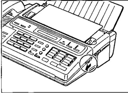
Slide the FRONT LID OPEN lever forward to open the document feeder unit.
