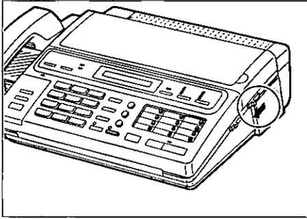
Slide the BACK LID OPEN lever forward to open the recording paper unit.
