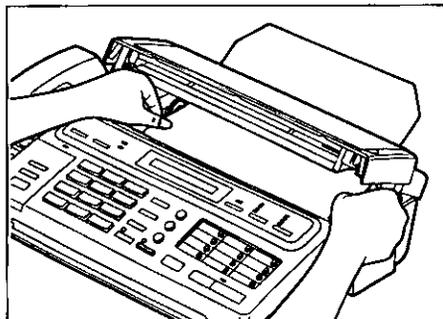
Then pull the paper a few centimeters (one or two inches) out of the unit.
