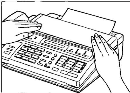
Close the paper compartment cover carefully by pressing down on both ends gently.
