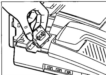
Insert the microcassette tape into the compartment with the full reel to the left. Make sure that there is no slack in the tape. Remove any slack by using a pencil and rotating the tape reel.
