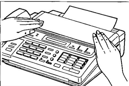
Close the recording paper unit carefully by pushing down on both ends gently.
