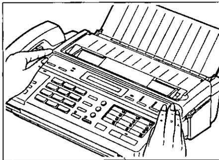
Then close the document feeder unit carefully by pushing down on both ends gently.
