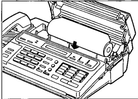
Place a recording paper roll into the paper compartment.
