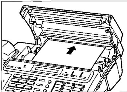
Insert the leading edge of recording paper into the recording paper exit.
