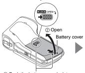
Push the battery cover lock to the right to release it. (a) Insert the battery pack (page 36), then close
