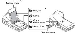
If the rubber seal inside the battery cover or terminal cover is cracked or deformed, consult the store where the camera was purchased or a nearby service center.
