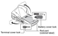
1 Check that there is no foreign matter on the inner side of the battery cover or terminal cover (where the rubber seal ① contacts the camera body ②).
