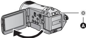
The status indicator **A** lights red and the unit is put into recording pause approx. 0.6 seconds after it is turned on.
