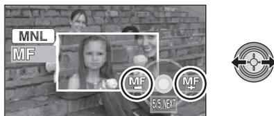
The center of the screen is enlarged. The normal screen returns approximately 2 seconds after you finish bringing the subject into focus.
