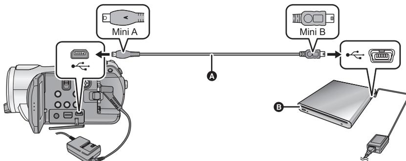
**A** Mini AB USB Connection Cable (supplied with VW-BN1)
