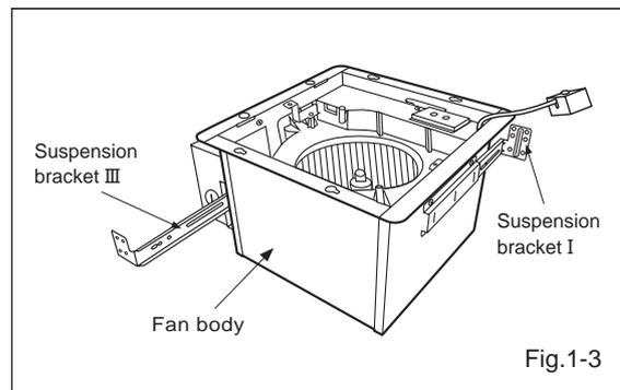
If spacing A on center joists is 24 inches, connect suspension bracket II and III (C4 mark to C4 mark) as shown below :
