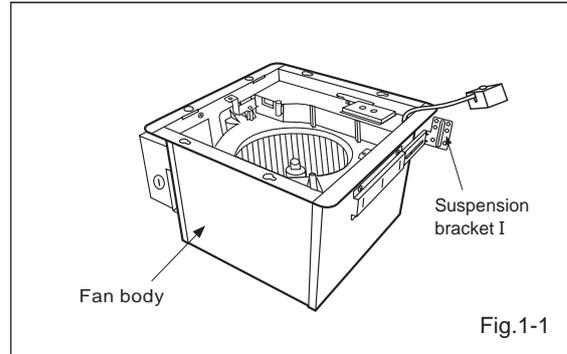
1. Insert the suspension bracket into the fan body and adaptor. (select the suspension bracket as shown below)
