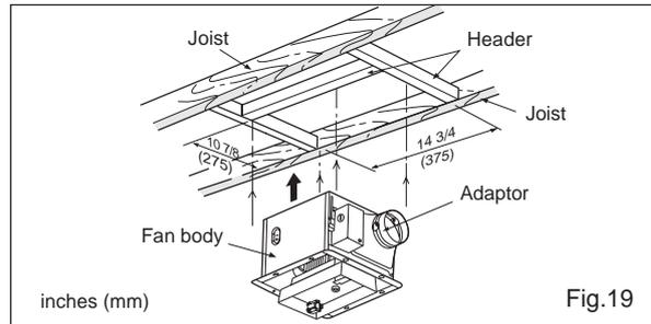
3. Install the fan body and secure it by using long screws (ST4.2X20) (Fig.19, Fig.20)
