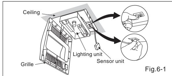
11. Insert the sensor unit into the housing of the grille and insert other mounting spring into the slot as shown and mount grille to fan body (FV-08VKML1) (Fig.6-2, Fig.6-3)
