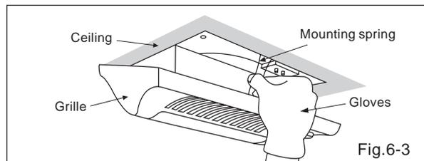
12. Insert mounting springs into the slots as shown and mount grille to fan body. (FV-08VKSL1) (Fig.7)
