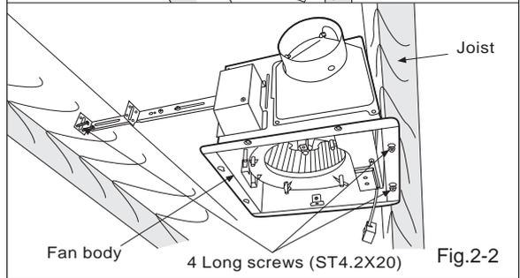
3. Install the suspension bracket to joists by using long screws (ST4.2X20) and secure it to the fan body by using screw II (ST4.2X12) (Fig.3)
