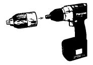
2 Inserting the bit Insert the bit, and turn the lock collar clockwise(looking from the front) holding the sleeve until laws close firmly
