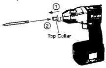
3 Removing the bit Pull the top collar of the Quick change chuck forward then pull the bit
