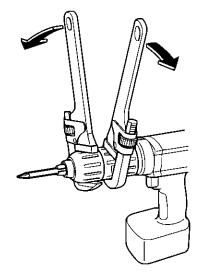
4 Detaching Keyless drill chuck To detach the chuck, PUSH the button to release the chuck from the square drive
