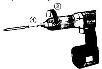
3 Removing the bit Turn the lock collar counterclockwise (looking from the front) Then remove the bit
