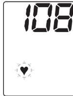
The heart mark ♥ will blink when pulse is detected during pressurization.
