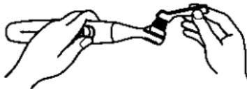
Push down the lock button and open the blade mechanism.
