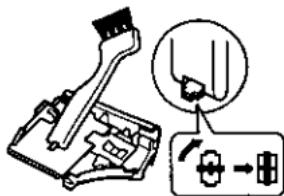
2. Remove the stationary blade and clean it and the moving blade.
