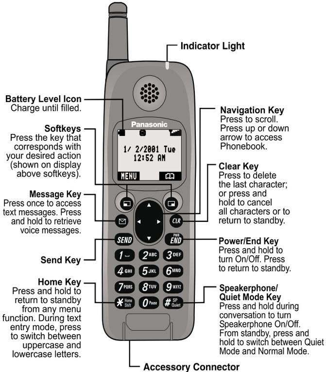
You may enter up to 32 characters by pressing the number keys. The keypad is also used to enter text as described in "Text Entry Operations", Chapter 4.
