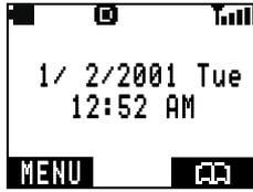
**MENU** shows on the bottom left side of the display. To access the Main Menu, press the corresponding softkey (☰) on the keypad just below where **MENU** is displayed. After entering the Main Menu, press either softkey (☰ or ☲) to select the options displayed above them.
