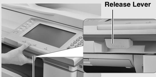
Pull the Release Lever to adjust the viewing angle.
