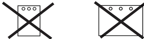
Also, when punching B5 □, A4 □, 8.5 x 11" □ size paper, check that the paper of □ orientation is loaded in the tray.
